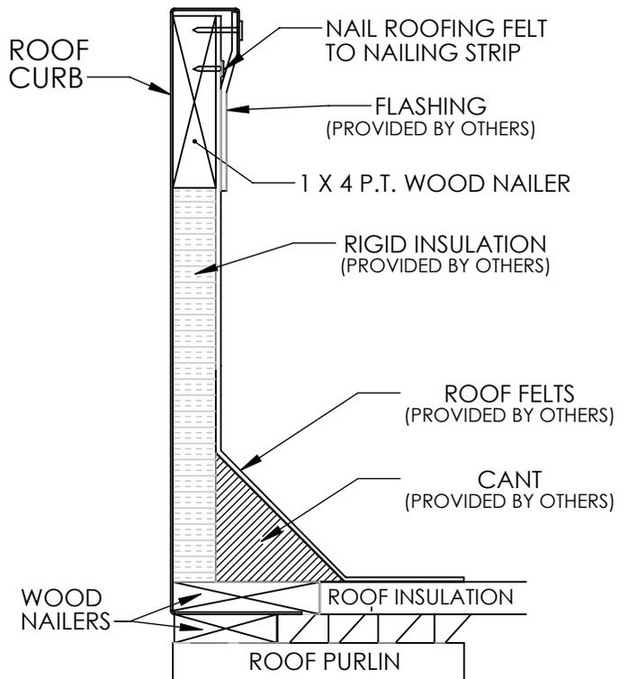
**FIGURE B - Typical Roof Curb
