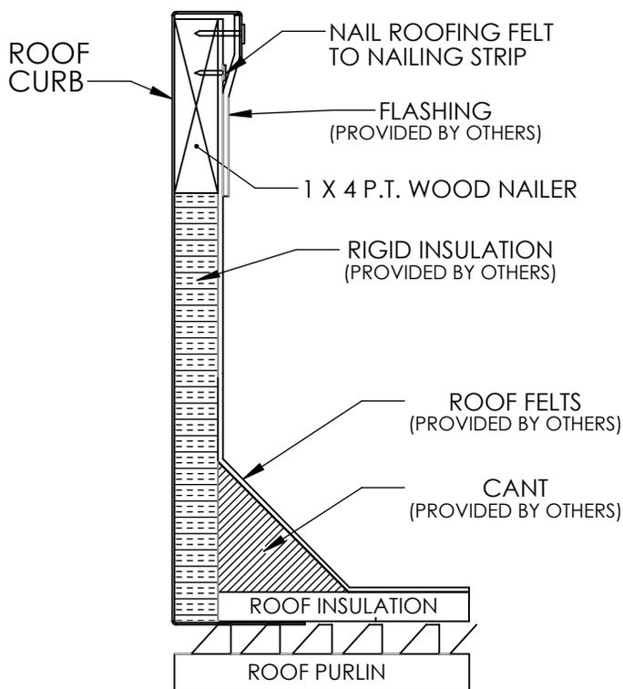
**FIGURE A - Typical Roof Curb
